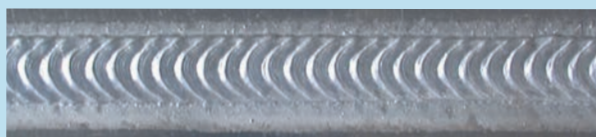
16 gauge (1.6 mm) A5052 Aluminum Plate Butt Welded With 3/64" (1.2 mm) A5356 Aluminum Wire
